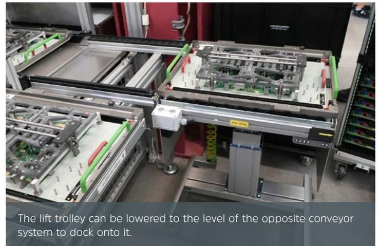
The lift trolley can be lowered to the level of the opposite conveyor system to dock onto it.
