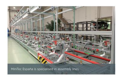
MiniTec España is specialised in conveying equipment and focuses on higher piece weights and assembly lines. A flexible assembly system (FAS) has now been further expanded for a customer in the automotive industry. One assembly line model has already been in use in multiple plants worldwide for 15 years. It is an FAS in the form of a horizontal circuit for the assembly of car instrument panels. The parts move on jigs designed and
