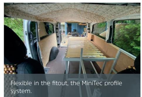
Flexible in the fitout, the MiniTec profile system.
