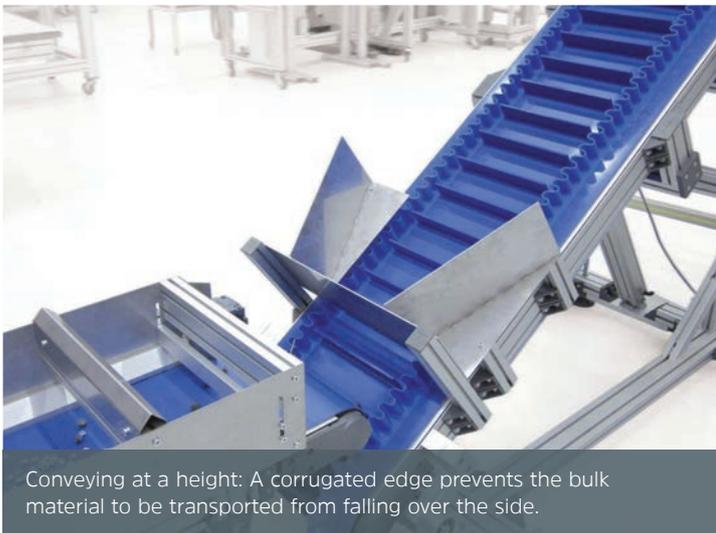
Conveying at a height: A corrugated edge prevents the bulk material to be transported from falling over the side.
