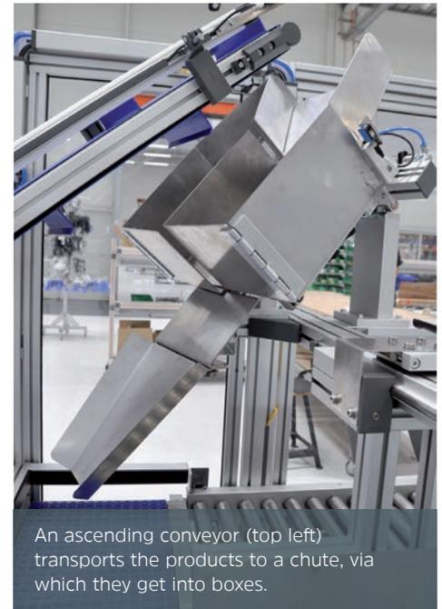
An ascending conveyor (top left) transports the products to a chute, via which they get into boxes.
