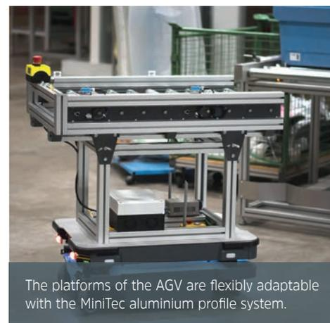
The platforms of the AGV are flexibly adaptable with the MiniTec aluminium profile system.
