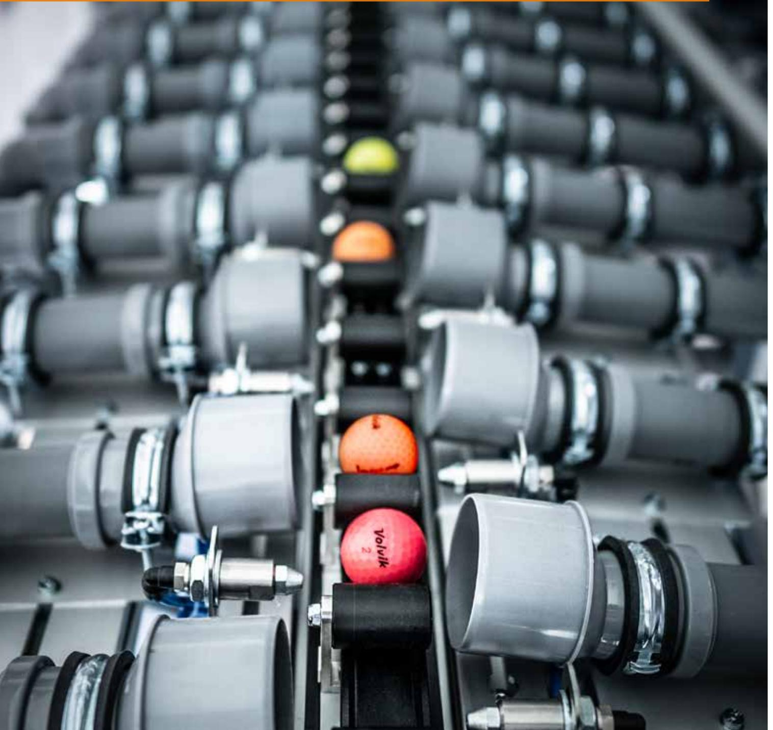
**Lake balls are used golf balls, which are recovered from bodies of water on golf courses, recycled and then placed on sale again. The Easy Lakeballs company in Wiesbaden is specialised in doing exactly that. It engaged Meprovision and MiniTec to produce a system which sorts the balls by brand and type with the help of AI.**
