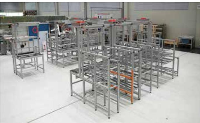
The U-shape of the system allows fluid, assembly in the team based on division of labour (task segmentation).
