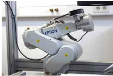
A 6-axis robot with magnetic grippers supplies the measuring station with parts.
