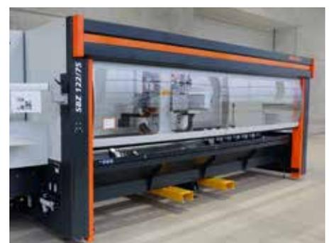
The new 5-axis machining centre enables complex profile machining.
