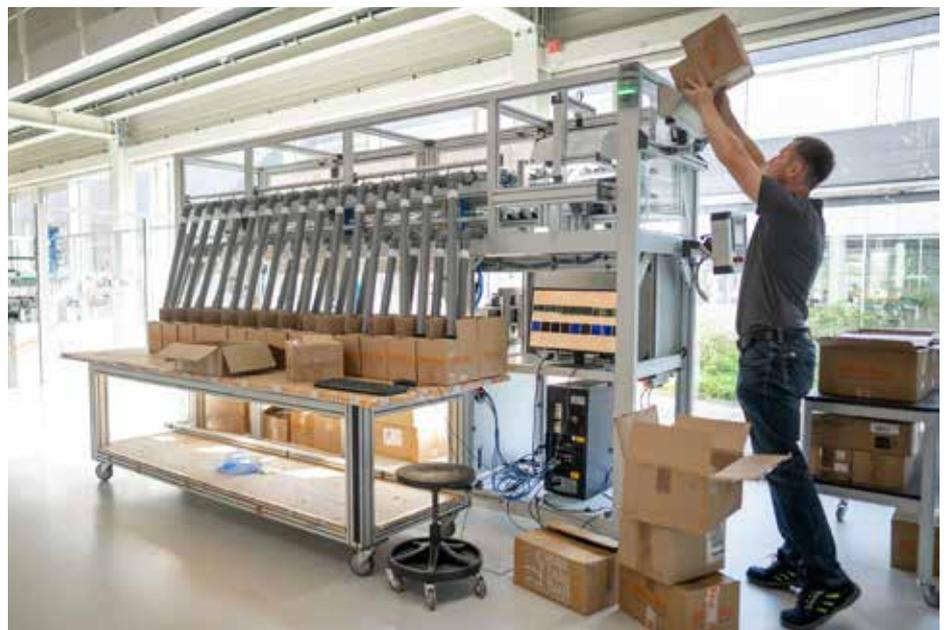
The system during the test run – a Meprovision employee fills it with golf balls. An automatic step conveyor will be used here later.
