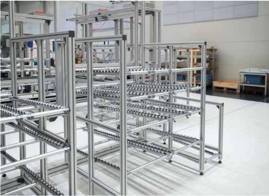
The material is supplied via kanban bins on roller strips from the back of the workstations.
