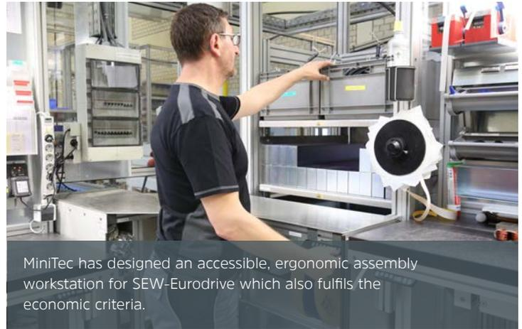
MiniTec has designed an accessible, ergonomic assembly workstation for SEW-Eurodrive which also fulfils the economic criteria.
